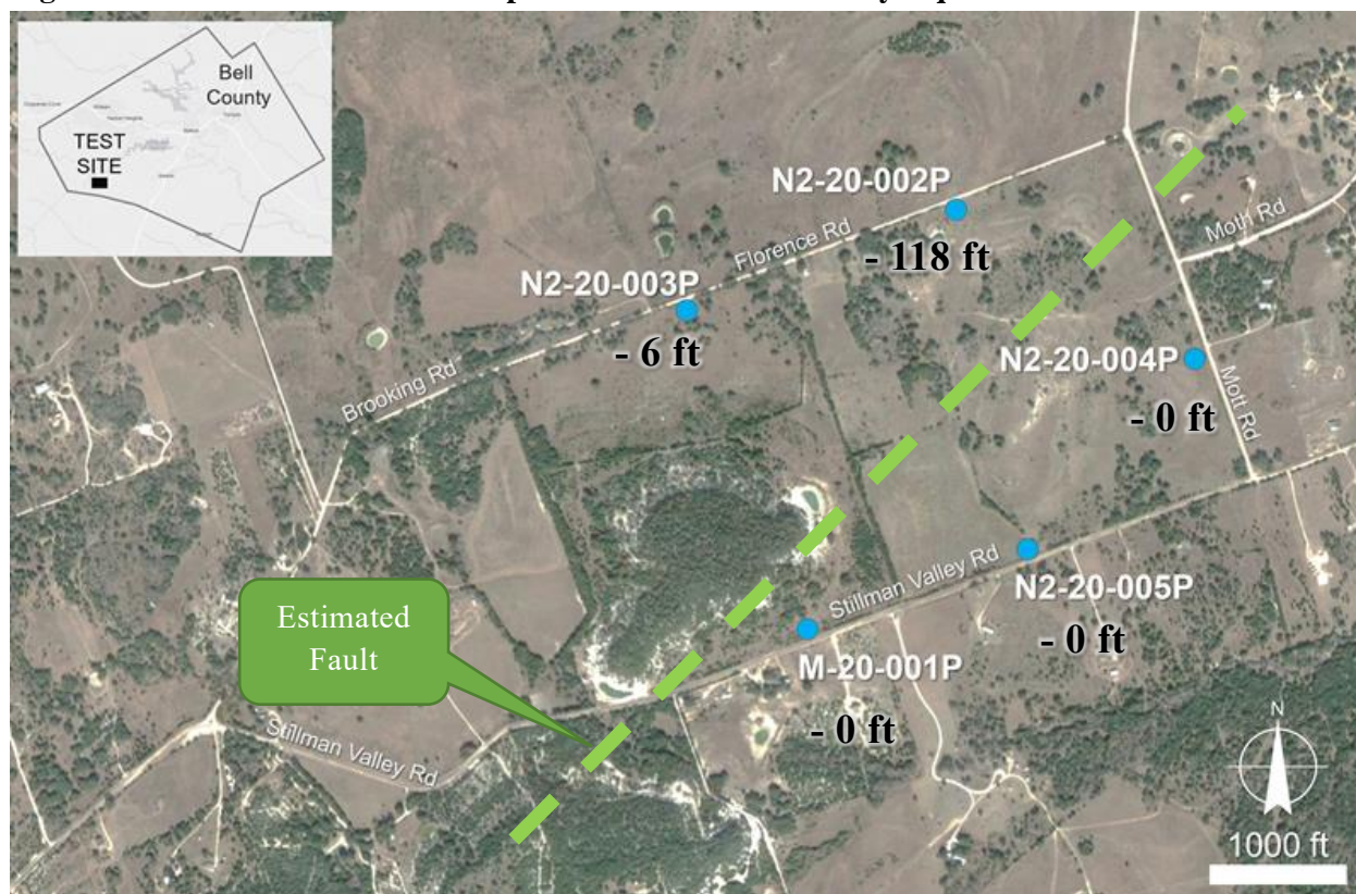
Figure 4. Drawdown in wells completed in the Lower Trinity Aquifer at the Hines site.
