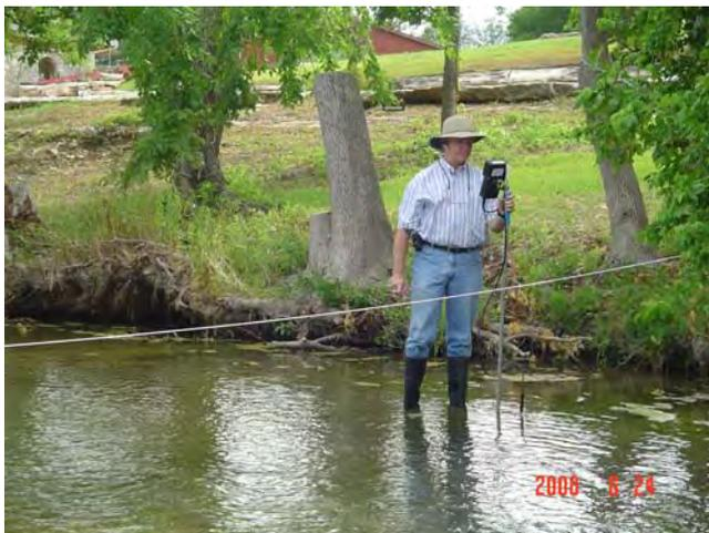
Measurement of stream flow in Salado Creek at lower gauge site in June 2008.
