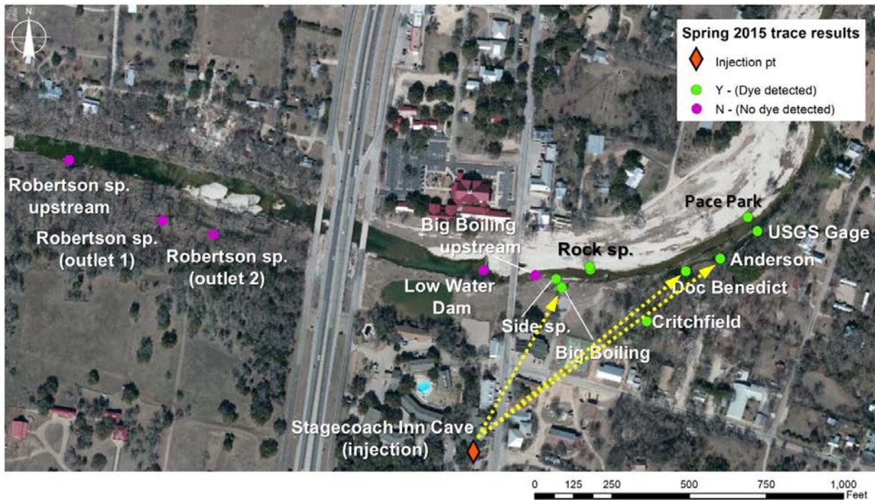
Figure 12: Results of the spring 2015 dye trace test. Purple dots indicate locations of no dye detection. Green dots indicate spring and creek locations where uranine was detected. Arrows represent confirmations of groundwater flow between the injection point at Stagecoach Inn Cave Well and a spring.
