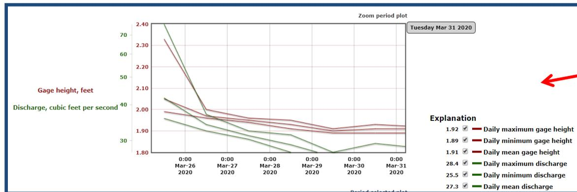
CFS is measured continuously at the downstream gage with USGS developing the rating curve according to industry standards and maintaining the information for public access on the USGS website.
