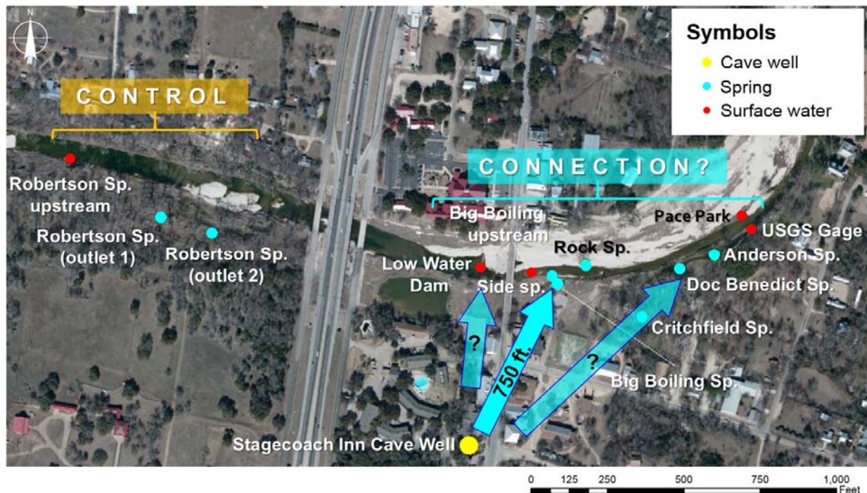
Figure 2: Conceptual overview of the Salado Springs dye trace test on April 18, 2015.
