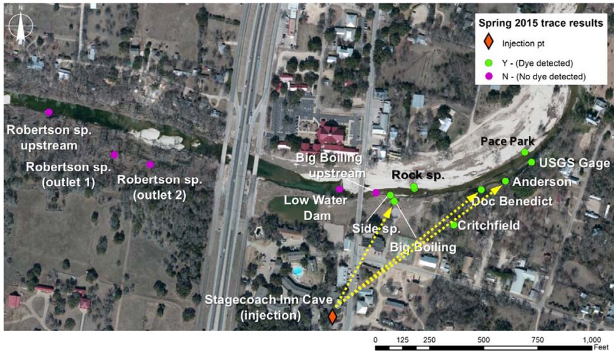
Figure 3: Results of the spring 2015 dye trace test. Purple dots indicate locations of no dye detection. Green dots indicate spring and creek locations where uranine was detected. Arrows represent confirmations of groundwater flow between the injection point at Stagecoach Inn Cave Well and a spring.
